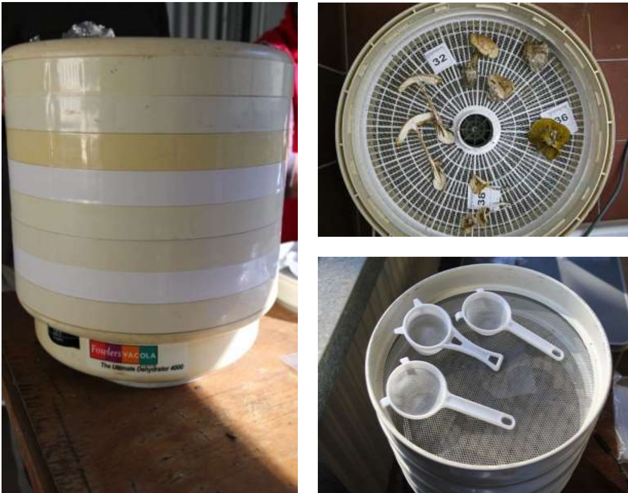
Figure 13 Food dehydrator (left) with large fungi (top right) and ready for small fungi (bottom right). These can be bought for as little as $40 – the only mandatory feature is some form of temperature regulator.
